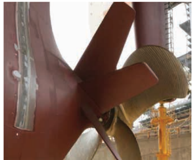
Figure 10. Stators on CMA-CGM Containership CHRISTOPHE COLOMB
