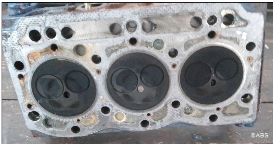
Inoperative freefall lifeboat engine/unit dismantled for overhaul
