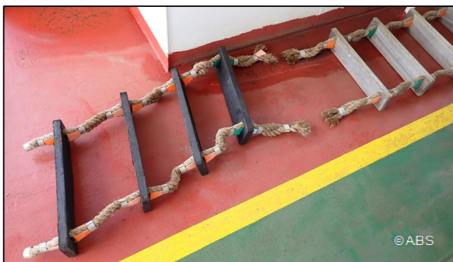
Damaged pilot ladder – rope parted both sides while pilot on the ladder due to wasted rope
