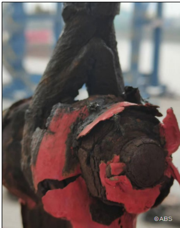
Rescue boat release hook shackle wasted with rust
