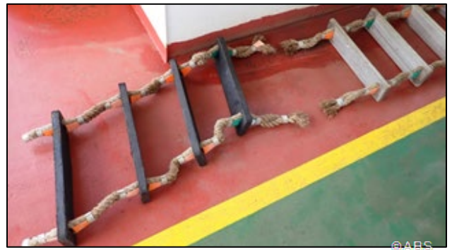
Damaged pilot ladder- rope parted both sides while pilot on the ladder
