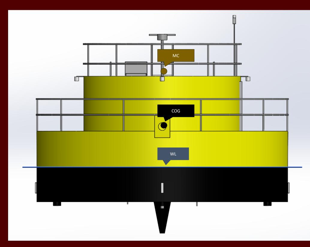
Buoy Weight: 125 Tons
