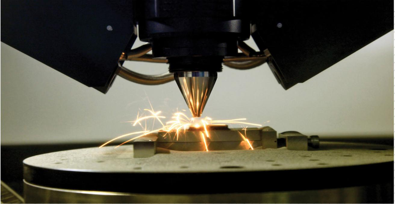
Additive manufacturing (AM), or 3D printing, refers to multiple manufacturing processes that build parts by adding material layer-by-layer, thereby replacing or augmenting more traditional manufacturing processes such as casting and forging. AM can shrink the supply chain and lead times for specialized and complex parts, introducing new efficiencies driven by design innovation, reduced manufacturing time, and improvements in part availability.
