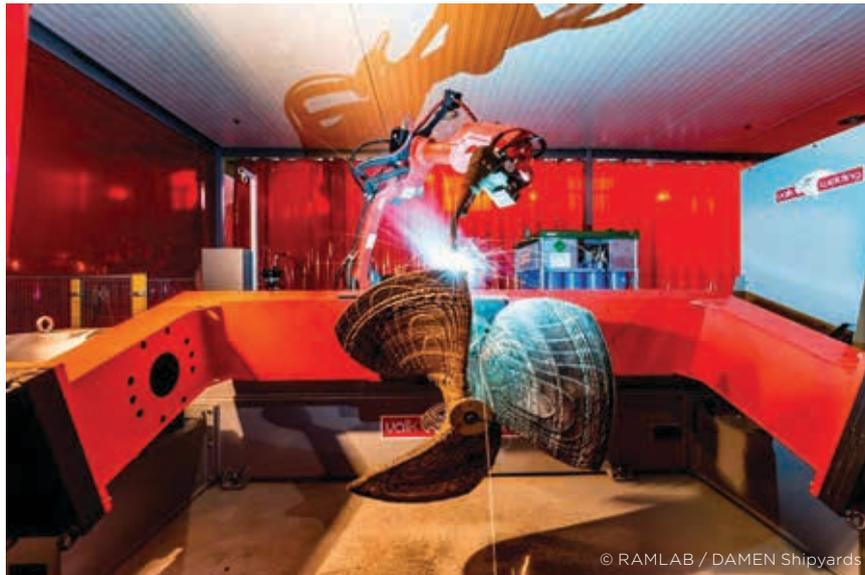
*Figure 2 – Additively manufactured propeller*
