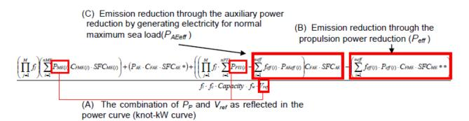
The MEPC.1/Circ. 815 Guidance categorizes Innovative Energy Efficiency Technologies into 3 categories based their characteristics and effects on the EEDI formula. Air lubrication is classified as Category B-1 for technologies that reduce the propulsion power but do not generate electricity and can be used at any time during vessel's operation. In effect, the power reduction is through adjustment to the 5<sup>th</sup> term in the numerator of the EEDI formula.
