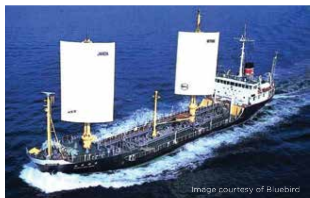
Vessel Shin Aitoku Maru with rigid sails
