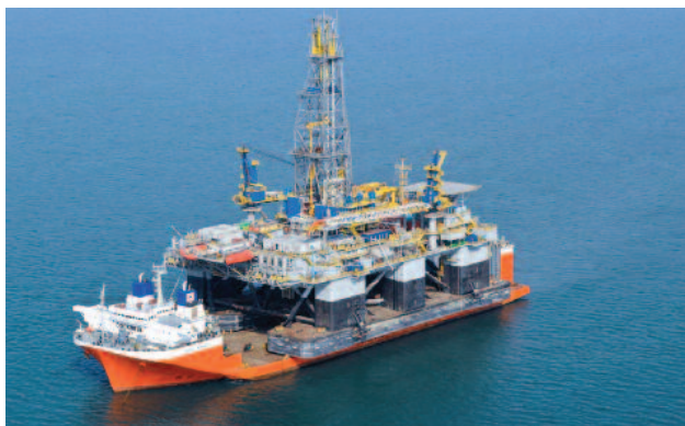
DSIC delivered the ABS-classed Noble Dave Beard sixth-generation semisubmersible, shown here aboard the Dockwise Mighty Servant 1 transport vessel in 2009. (Source: DSIC)
