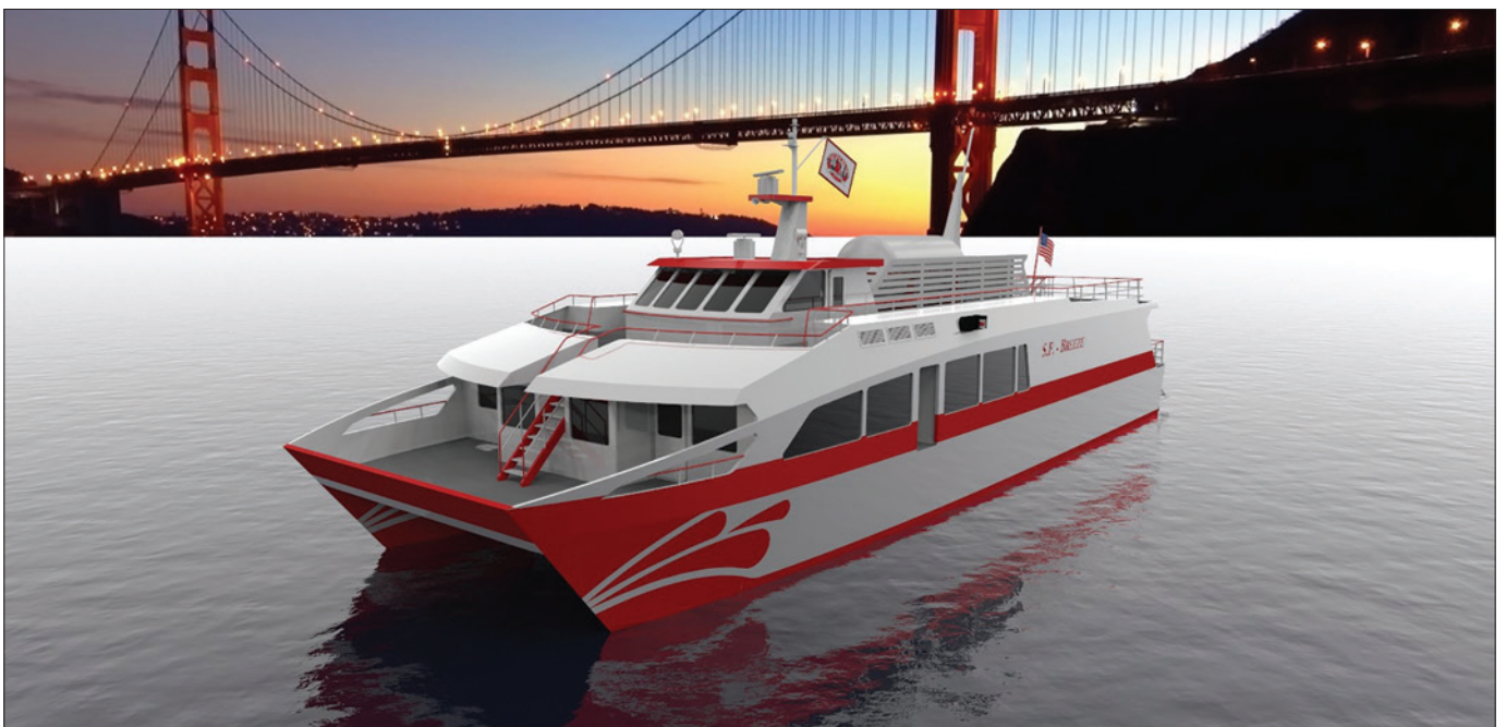
The SF-Breeze — designed to complete four 50-mile round trips each day...with zero emissions.
