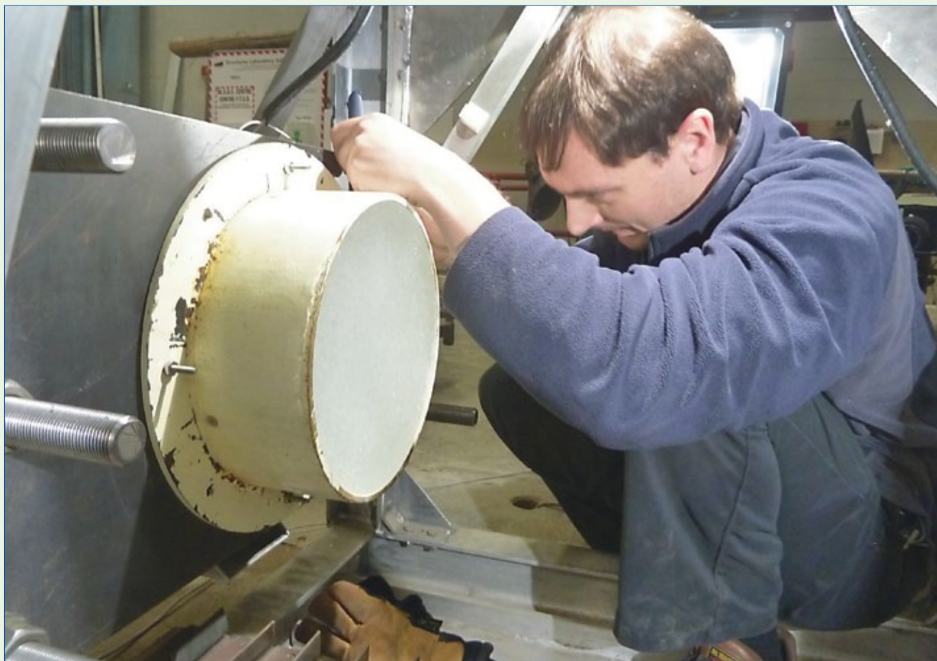
ABS HETC engineer prepares ice sample for dynamic ice-crushing test.
