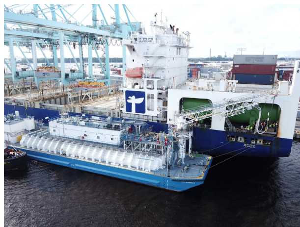
Figure 3. Clean Jacksonville , owned by TOTE Maritime, has been used for bunkering TOTE's two 3100 TEU, Marlin-class containerships (credit: GTT).
