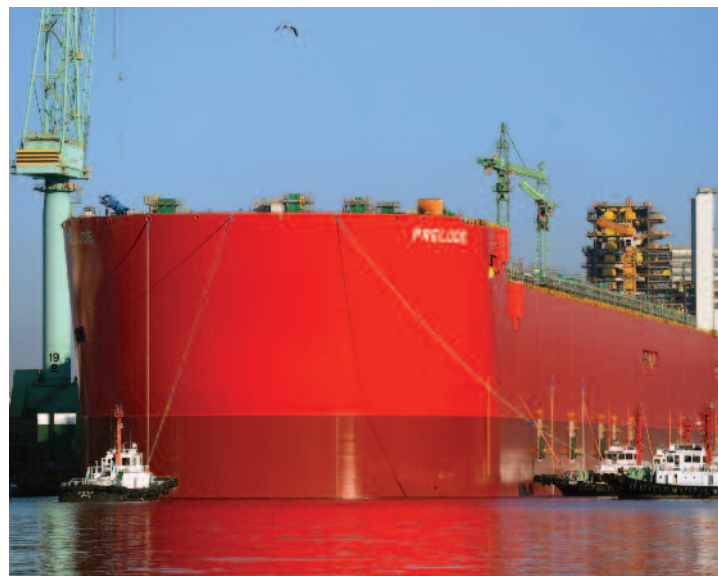
The Prelude hull was completed and floated from the drydock in November 2013. Nine tugboats were required to move the 488-m long hull. (Image courtesy of Shell)
