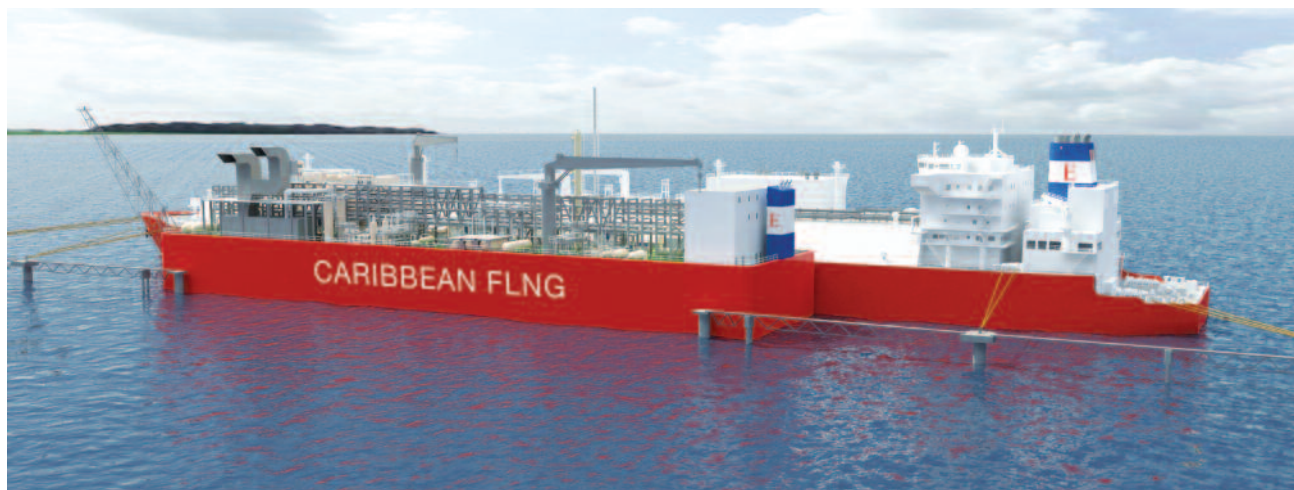
The artist's rendition of the Caribbean FLNG facility shows an LNG carrier docked next to the liquefaction barge. Caribbean FLNG will begin commercial production in 2Q 2015. (Image courtesy of EXMAR Marine)
