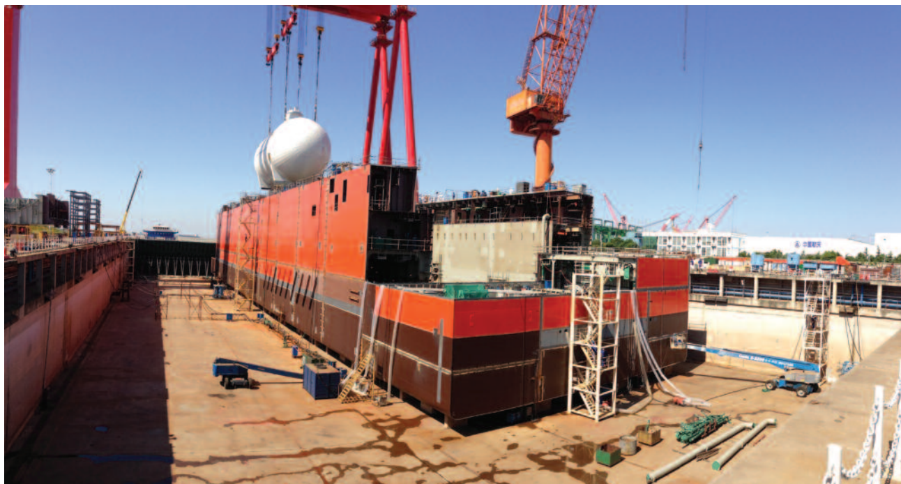
The cargo storage tank is lowered into the hull of the Caribbean FLNG barge at Wison Heavy Industry's shipyard in Nantong, China. (Image courtesy of EXMAR Marine)
