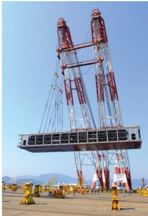
The keel was completed in May 2013, and Samsung began assembling the hull. A hull section is being lowered into place. (Image courtesy of Shell)
