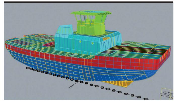
The software-agnostic goal was built into the work scope for the Crowley/Jensen pilot. It included the identification of 3D model formats that Jensen Maritime wanted to submit for ABS review, and the determination of the 3D models that were to be submitted for testing. The program was tested with hull scantling models. As the focus was on the plan-review workflow, a full engineering plan review of the models was not conducted for this part of the pilot.
