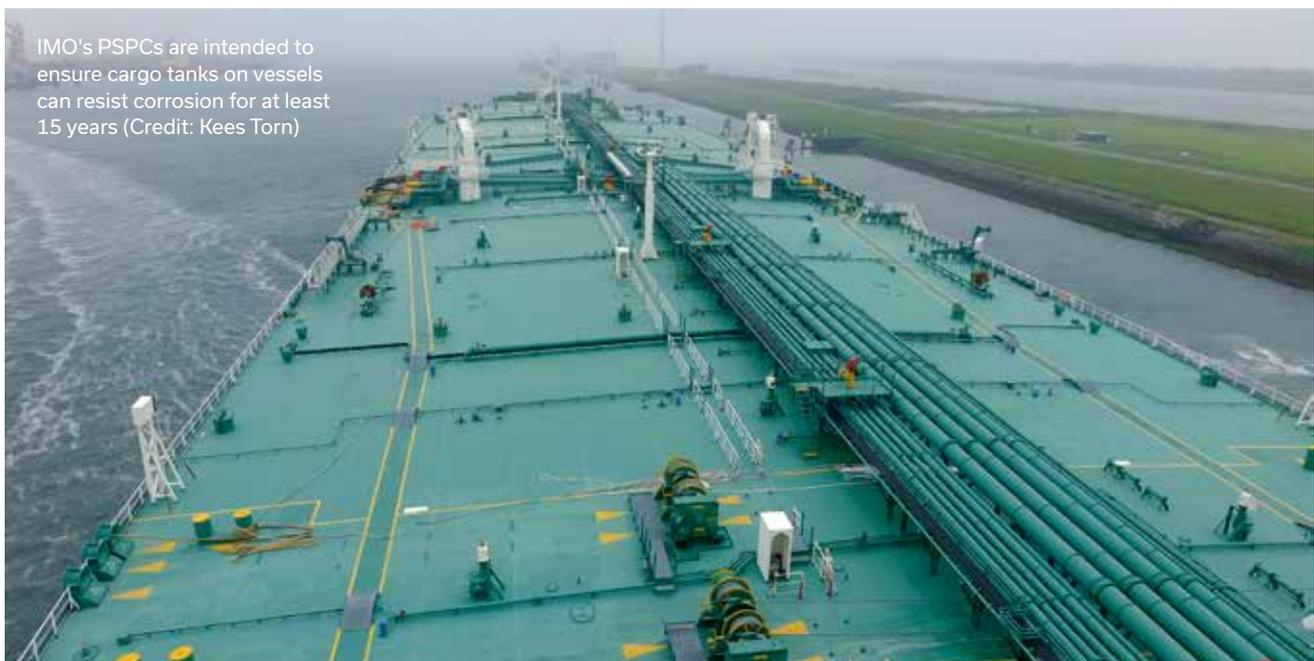
IMO's PSPCs are intended to ensure cargo tanks on vessels can resist corrosion for at least 15 years (Credit: Kees Torn)
