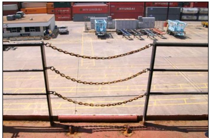
Handrail heights for safety at deck edges can vary depending on what ship design standard is selected. Design dimensions have traditionally accommodated the lower limit required, 39 inches (1000mm); however, it has recently been recommended that 39 inches (1000mm) is insufficient. The general opinion of safety engineers is that the lower limit is no longer adequate to deter falls over a rail for the 95th%
