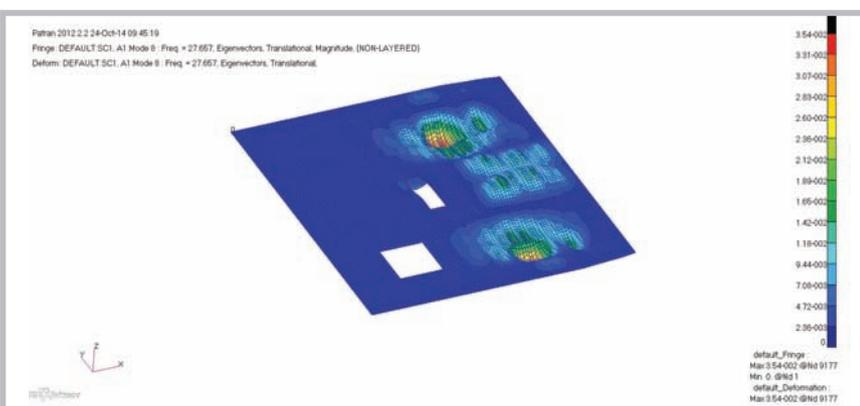
**SIRC teams created Finite Element Analysis models for free vibration analysis of a ship. The deformation shows the deck's natural vibration modes.**
