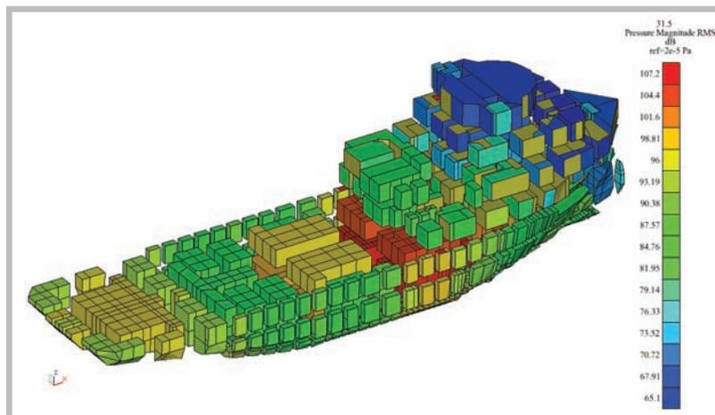
This SEA model was used for noise prediction on a ship. All images are courtesy ABS
