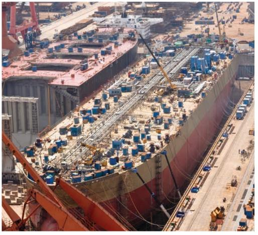
With the passage of OPA 90, double hulls were required for newly built tankers trading to the United States.
