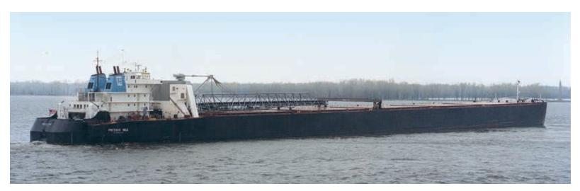
Designed for operating in the US Great Lakes, the PRESQUE ISLE is an integrated tug and barge combination that measures nearly 1,000 feet long.
