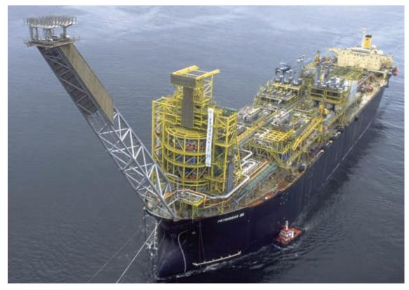
The PETROBRAS 35 floating production offloading and storage facility was converted from an ABS-classed tanker, the JOSE BONIFACIO.
