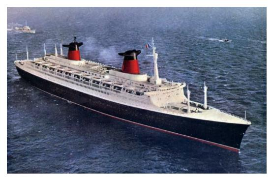
With an overall length of 1,035 feet, the ABS-classed SS FRANCE was announced as the world's longest liner when it was launched in 1960. This vessel also used aluminum extensively in its superstructure.
