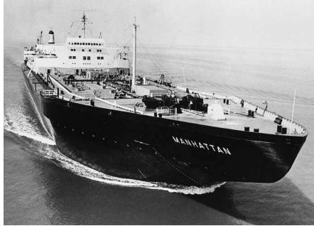
The tanker SS MANHATTAN, with special ABS-approved structural changes, demonstrated its icebreaking capabilities by crossing the Northwest Passage.
