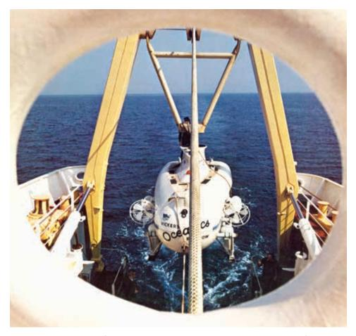
The VICKERS OCEANICS P. III, after completing a diving assignment, swings inboard at the stern of the mother ship. The manned submersible had two battery-powered electric motors and could dive to a 3,500-ft depth.
