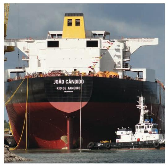
In 2010, the JOÃO CÂNDIDO was the first in a series of ten 160,000 dwt suezmax tankers built at Brazil's Atlântico Sul Shipyard for Petrobras' transport subsidiary, Transpetro.
