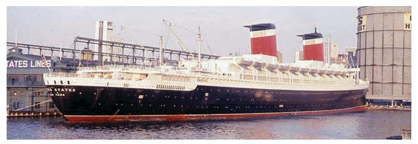
The beloved SS UNITED STATES was the fastest ocean liner ever built. Its superstructure used more aluminum alloy than any ship at that time. This was challenging for the builders but provided extreme weight savings. Its 105-ft beam could clear the Panama Canal locks with just two feet to spare on either side.
