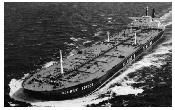
Measuring 1,244 feet in length, the 472,292-dwt GLOBTIK LONDON was the world's largest ship in 1973. It had a 93-foot draft and could make a service speed of 15.5 knots.
