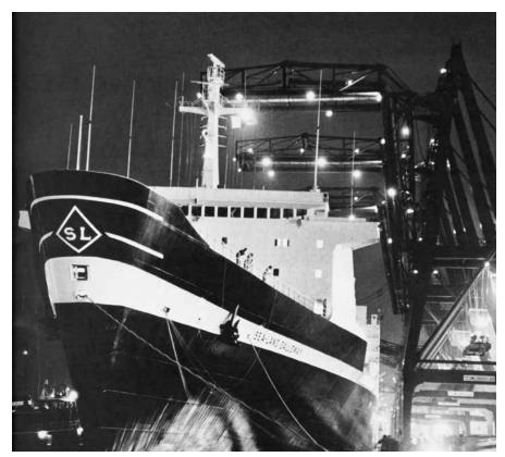
Sea-Land Service's SL-7 containerships were among the most advanced ships of the 1970s. There were eight high-speed, 27,358-dwt containerships of the same design, including the SEA-LAND GALLOWAY, with a twin-screw turbine drive and an operating speed of 33 knots.
