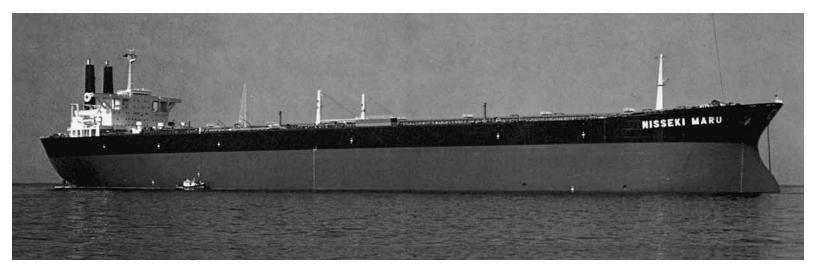
In 1971, the 366,812-dwt NISSEKI MARU was the largest tanker in the world. It was nearly 1,138 feet long with a beam of 180 feet.
