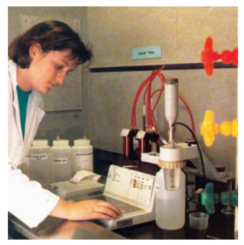
A laboratory technician with ABS Fuel Oil Testing operates an automatic titration unit to determine if the used lubricating oil contains excessive acid.
