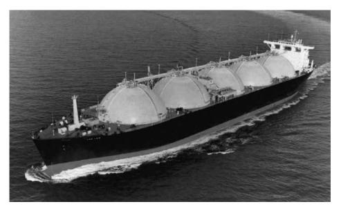
During the 1970s, the General Dynamics shipyard delivered a ten-ship series of 125,000 m<sup>3</sup> LNG carriers, produced with assistance from the DAISY program, including the 936-foot, ABS-classed LNG LEO.
