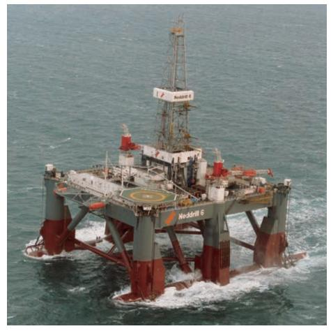
Delivered in 1981, the NEDDRILL 6 column-stabilized drilling unit operates today as the NOBLE TON VAN LANGEVELD.
