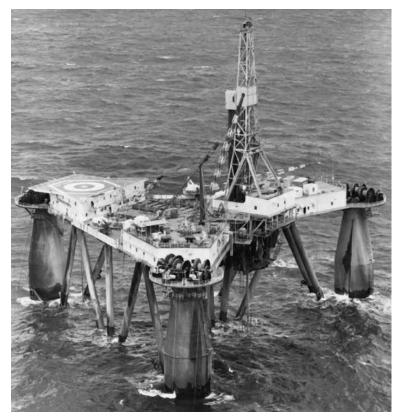
Friede and Goldman's SEDCO 135, the first purpose-built semisubmersible drilling unit. The design became internationally popular with its milk-bottle inspired legs.
