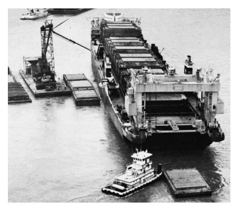
Special 60-foot barges are quickly stowed on a lighter aboard ship (LASH) vessel.
