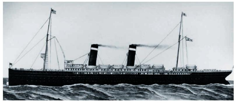
Launched in 1894, the SS ST. LOUIS was a transatlantic passenger liner built by William Cramp & Sons Shipbuilding and Engine Company in Philadelphia. It had a length of 554 feet and propulsion machinery supplying 20,000 horsepower.
