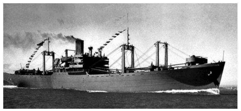
The USS JOHN LAND, built to the Maritime Commission's C2 design, was 459 ft long with a displacement of 13,893 tons and a steam turbine propulsion unit of 6,600 shaft horsepower.
