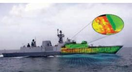
corroded condition using vessel gauging reports and experienced sea loading. This provides guidance on areas that need repair or require enhanced monitoring at specified inspection intervals.
