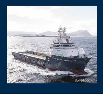
The ABS-classed SEACOR Yangtze is the company's first battery hybrid vessel capable of closed bus DP operations.
