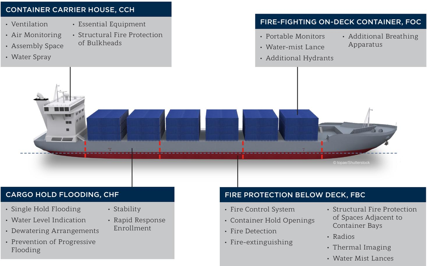
beyond what is required by the IMO. The guide supports enhanced fire- main piping arrangements and increased water supply by outlining requirements for additional equipment and arrangements that improve the vessel's firefighting capability.
