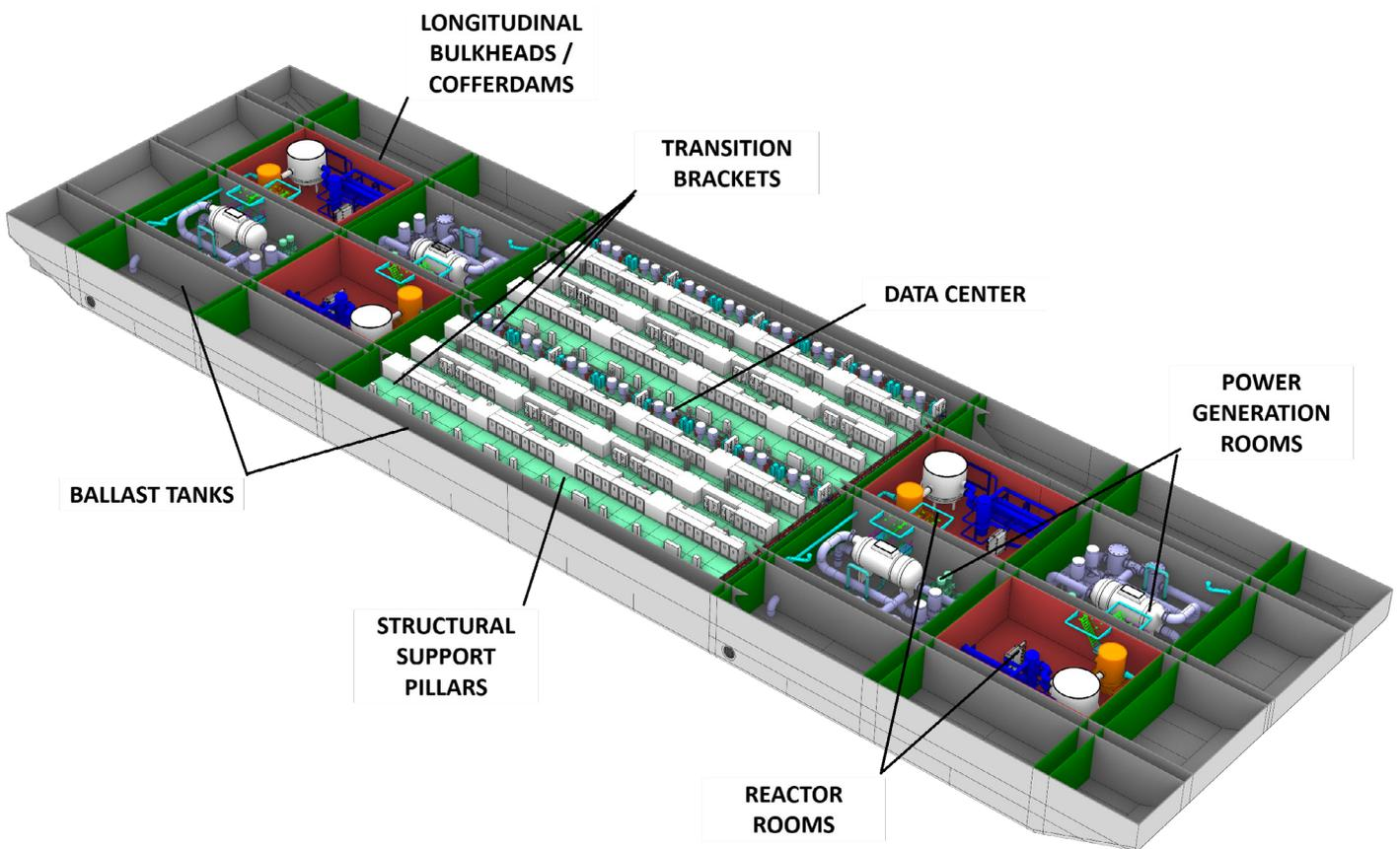
Figure 2: 22.5m ABL cut view depicting the layout and location of rooms and cofferdams.
