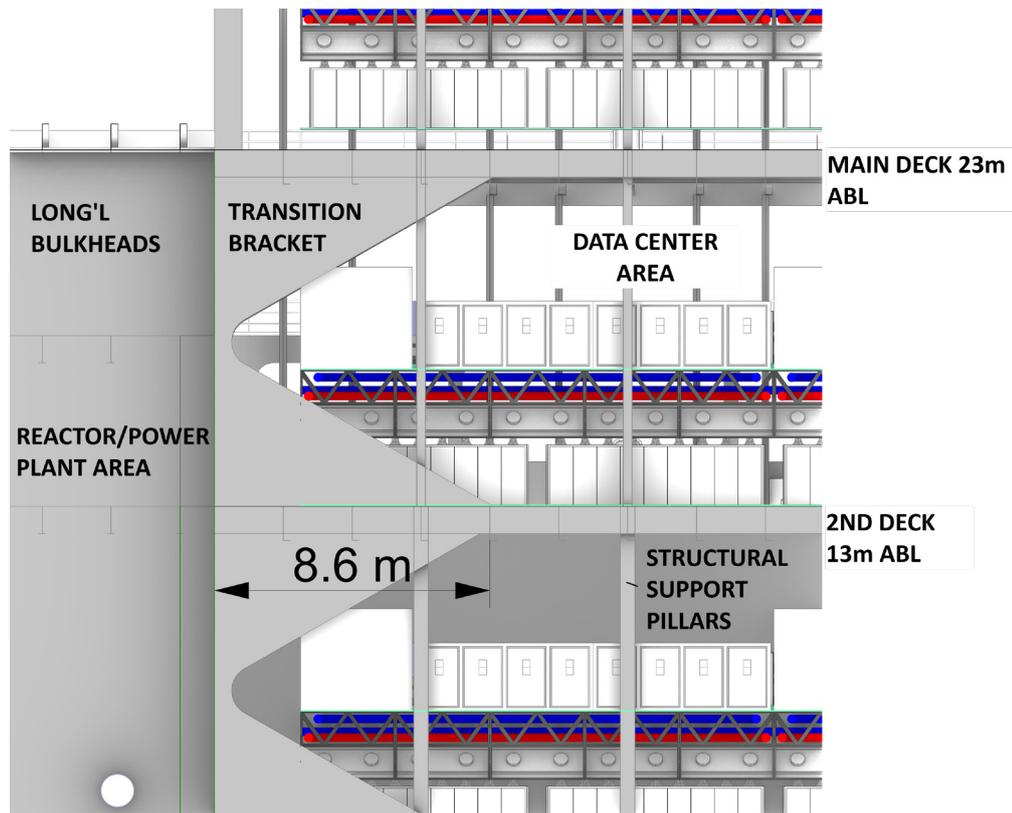
Figure 3: Longitudinal elevation at CL of transitional brackets between nuclear power plant and data center section.
