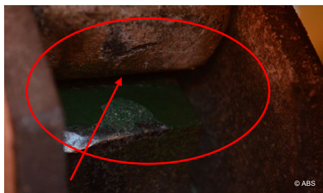
Freefall lifeboat release system defective (catch engaged) – before
