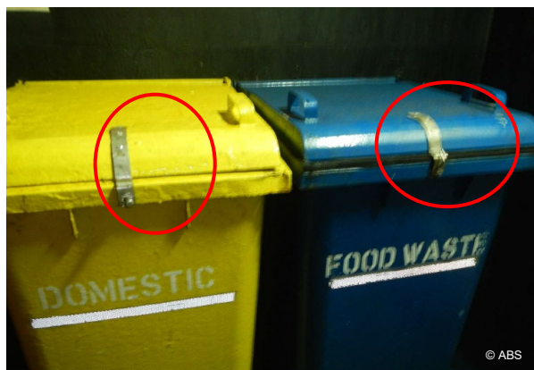
New fabricated securing device on cover of garbage receptacle
