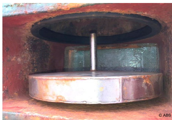
Forepeak tank air pipe found damaged replaced
