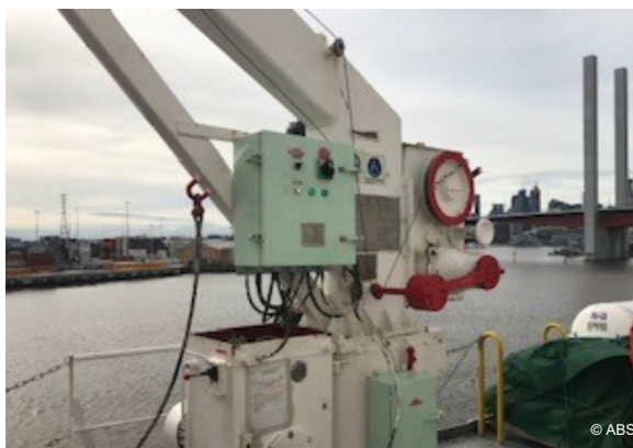
Rescue boat accumulator unable to maintain pressure
