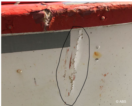
Lifeboat fractured on gunnel/side shell
