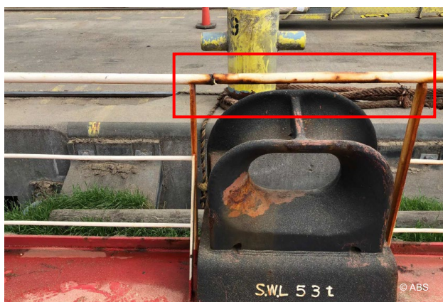
Handrail top tier found fractured
