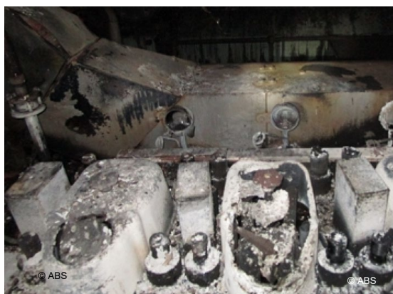
Damage to generator prime mover after fire
