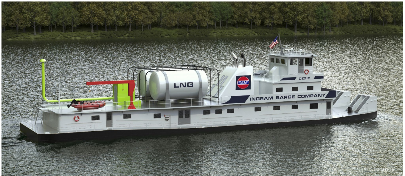
Figure 21. Mock photo of LNG retrofit application on an inland towboat. Mock image prepared for Ingram Barge by CT Marine (courtesy of Ingram Barge Company).
