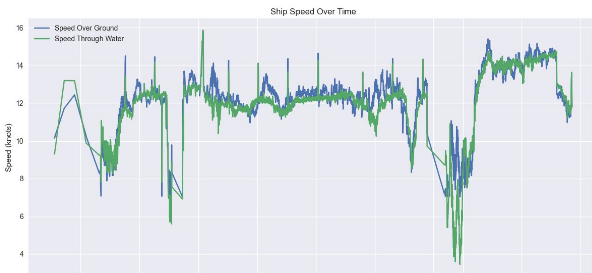
Figure 1: Example of measurements analysis: Speed Over Ground versus Speed Through Water. Significant deviations indicate data that should be filtered out from vessel performance analyses.
