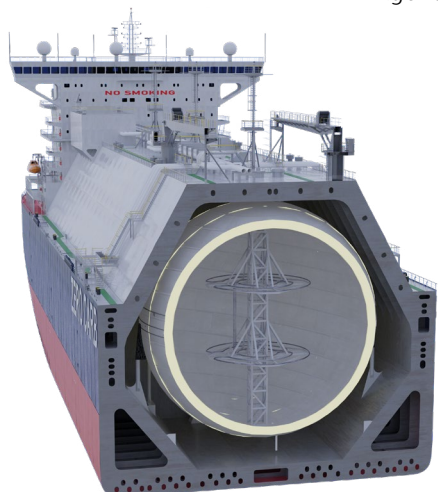
Figure 5.16: \text{LH}_2 carrier concept design rendering.
