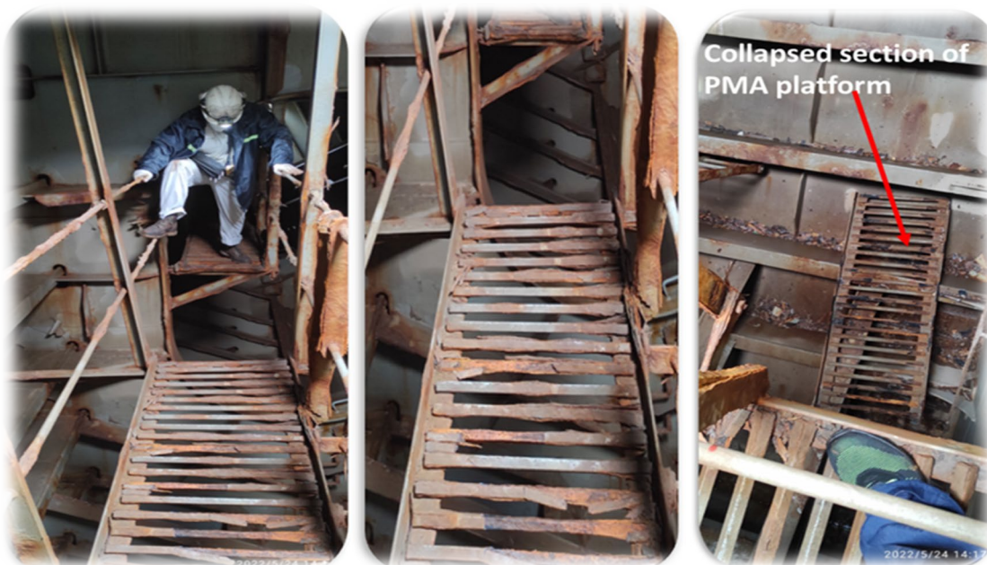
Figure 1. Collapse of PMA platform during inspections on 10-year-old Bulk Carrier.
