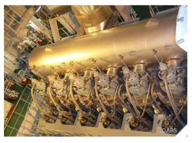
Where engines are intended for burning residual fuel oils, or other special fuel oils which may be interpreted as applicable to biofuels, the suitability for that is to be demonstrated during shipboard trials as per Marine Vessels Rules 4-2-1/13.9.6.
