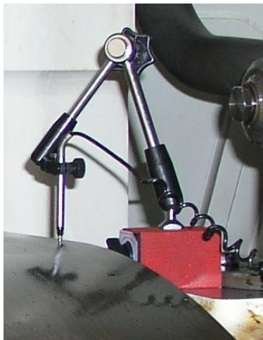
FIGURE 3 Reaction Measurement at Intermediate Shaft Bearing
