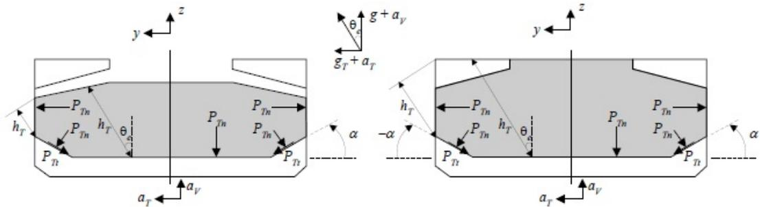
**5.3.3 Dynamic Bulk Cargo Pressure due to Longitudinal Acceleration**
