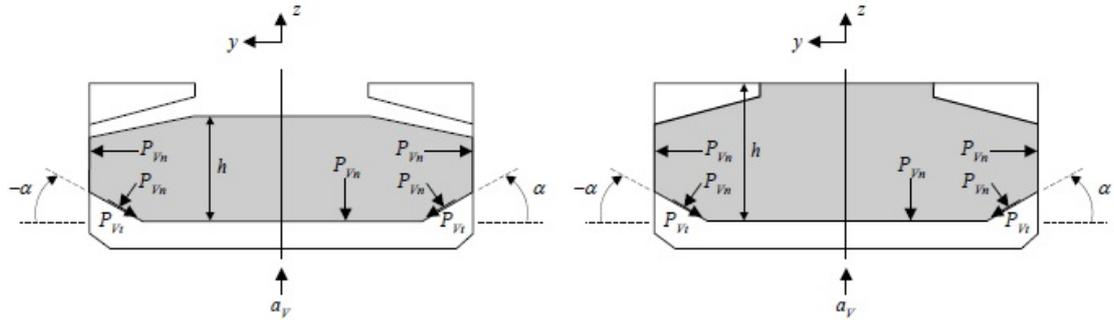
**5.3.2 Dynamic Bulk Cargo Pressure due to Transverse Acceleration**
