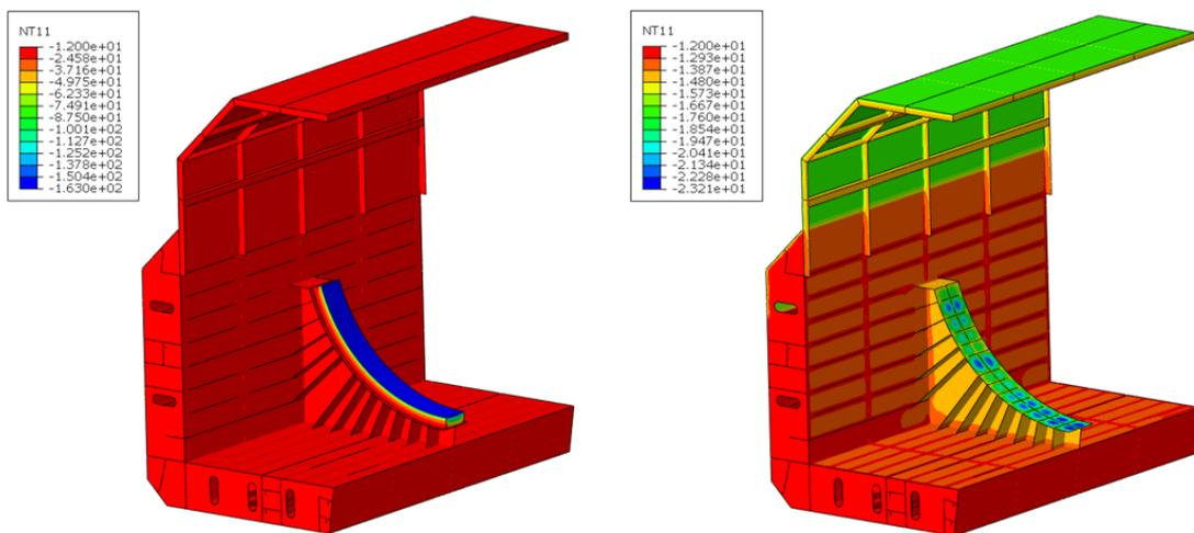
(B) Temperature Distributions of a Supporting Structure with Press-wood (Left) and without Press-wood (Right)
