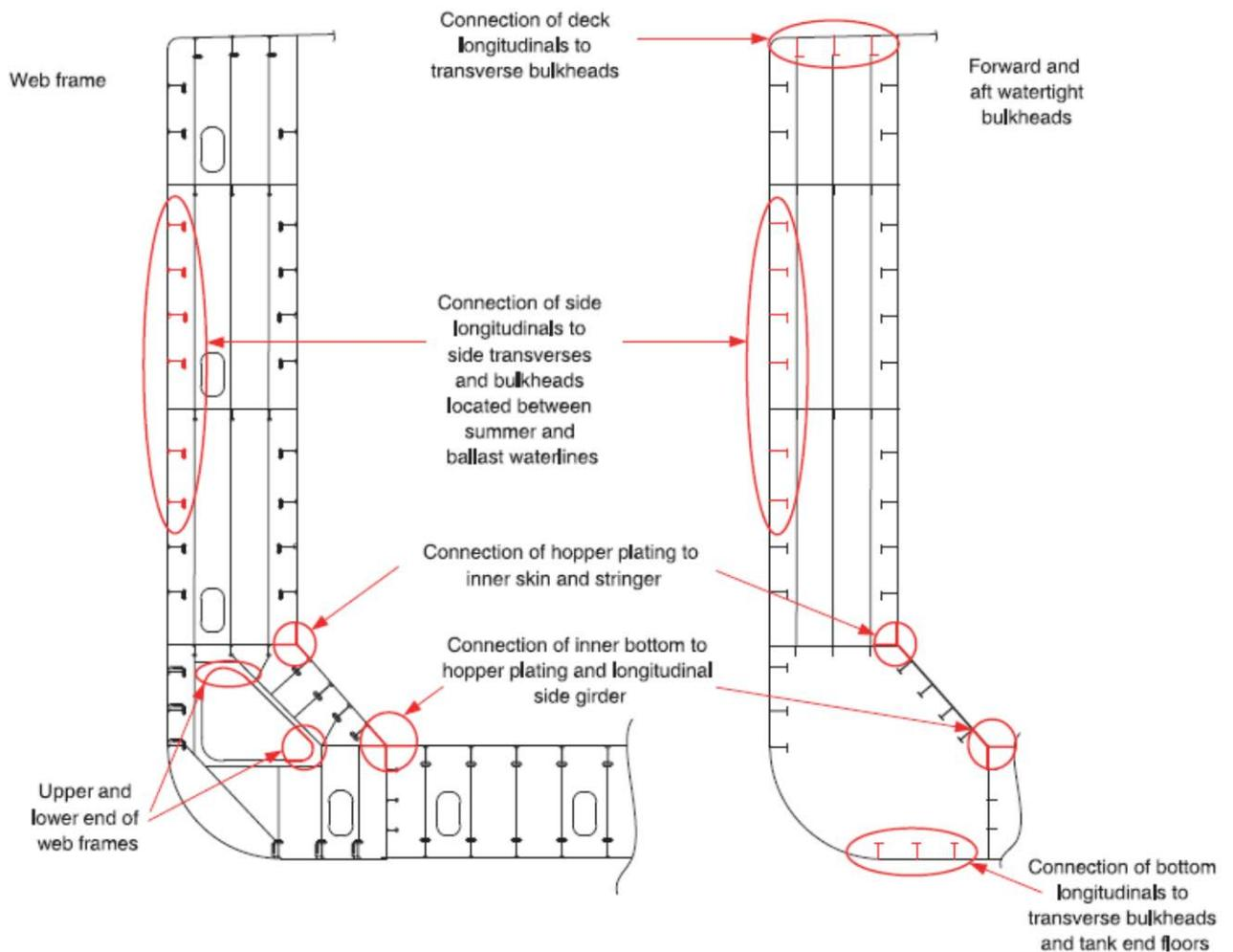
9.5 Critical Areas in a Single Hull Tanker
