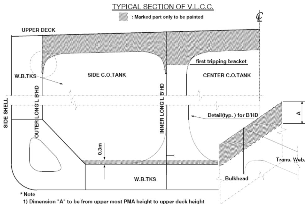
**3.3 Deck Head with Upper Transverses and Longitudinal Bulkheads**
