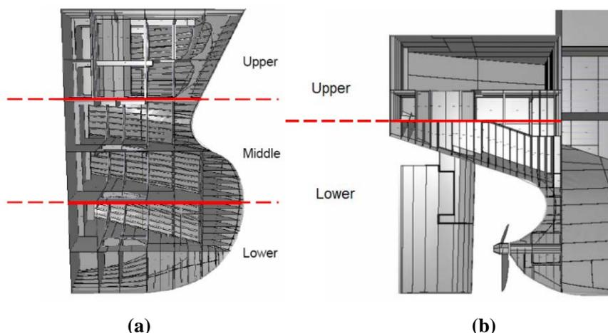
**7 Coated Areas of Ballast Tanks in Vessels other than Oil Tankers**
