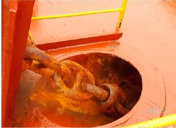
Anchor chain swivel worn out- port side
