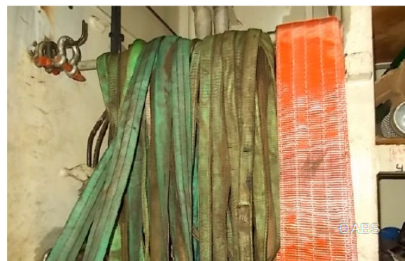
Safe operating marking missing for slings
