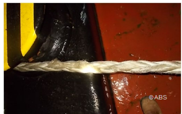
Frayed mooring lines
