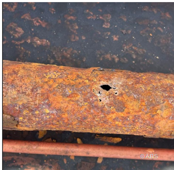
DECK CONDUIT PIPE WASTED
