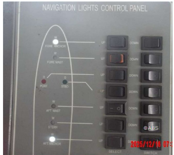
The aft mast light and forward anchor light are out of order.
