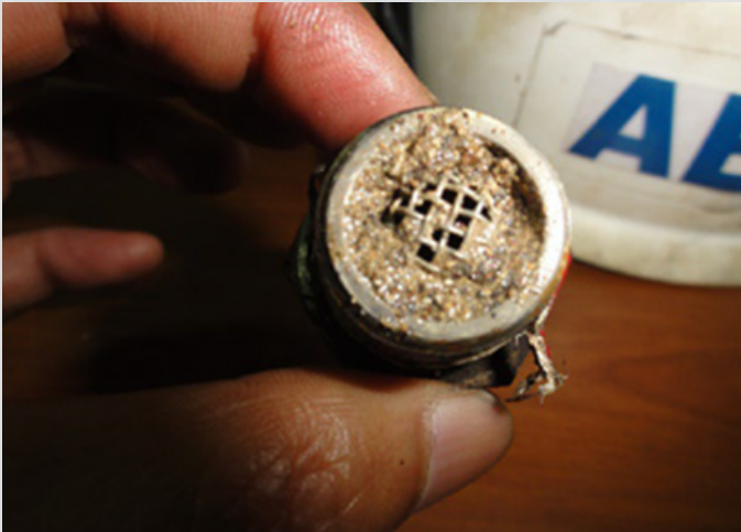
Water mist flexi fog system nozzle clogged
