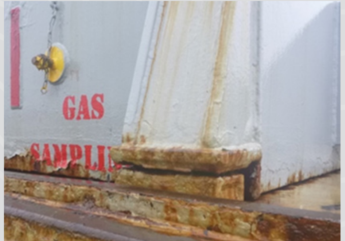
Hatch cover support pads with excessive wear, over compressed weathertight gasket and panels resting on coaming
