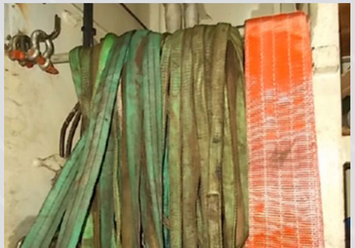
Safe operating load markings missing for slings
