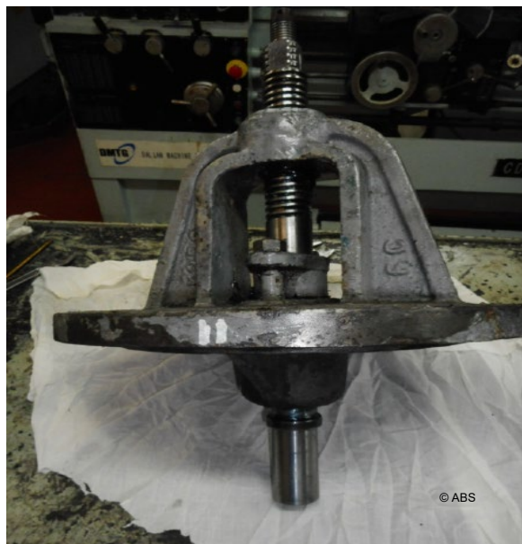
Emergency bilge suction overboard pipe – after maintenance
