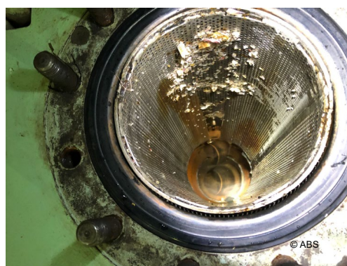
Main lubrication oil cooler with strainer free from ice - after
