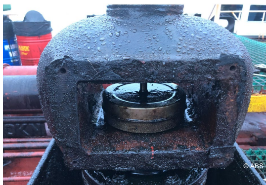
Fuel oil tank air pipe after cleaning
