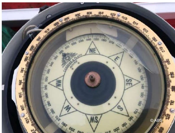
Magnetic compass with air bulb and light not working
