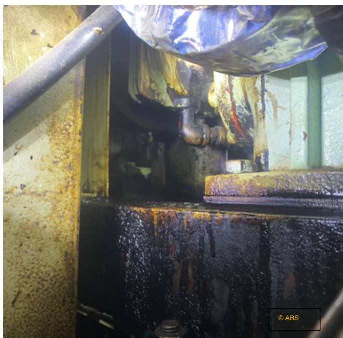
Leaking fuel oil pump
