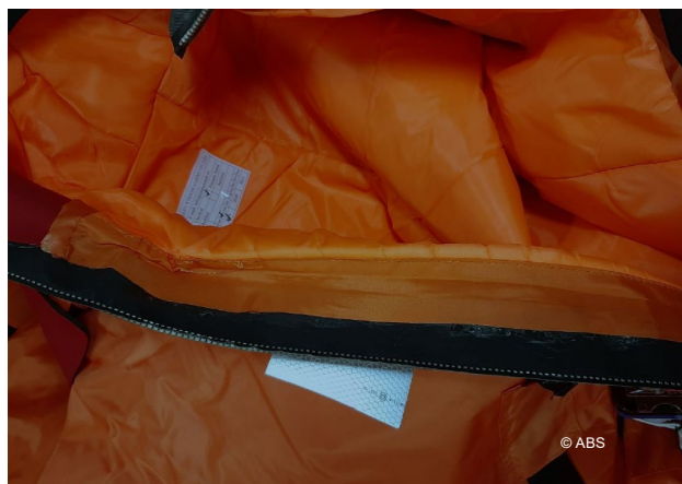
Immersion suits - glued parts detached
