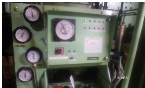
Main engine remote propulsion control (servo motor) malfunctioned
