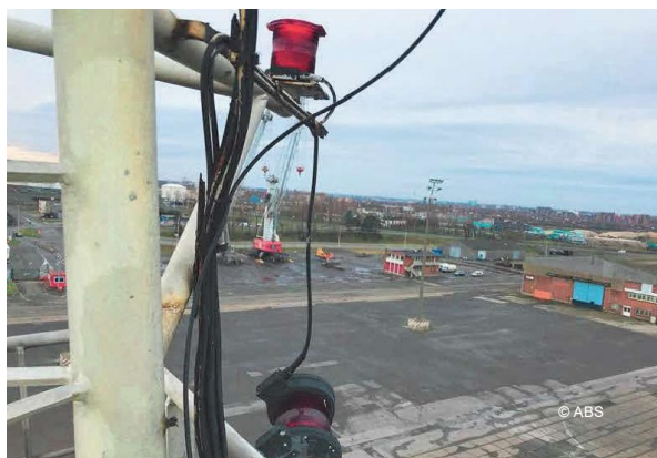
Navigation lights on mast found detached
