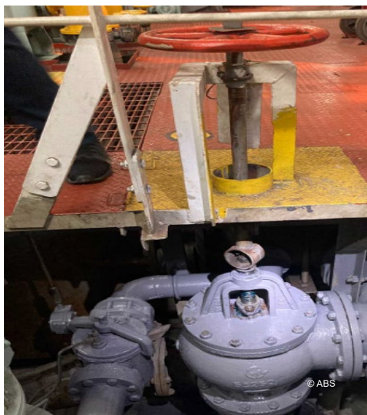
Emergency bilge suction overboard pipe – stuck valve
