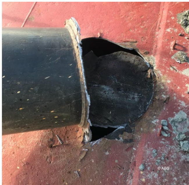
Damage to the main deck under a fairlead roller in way of anchor windlass
