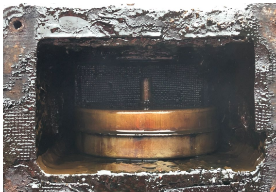
Fuel oil tank air pipe before cleaning due to overflow
