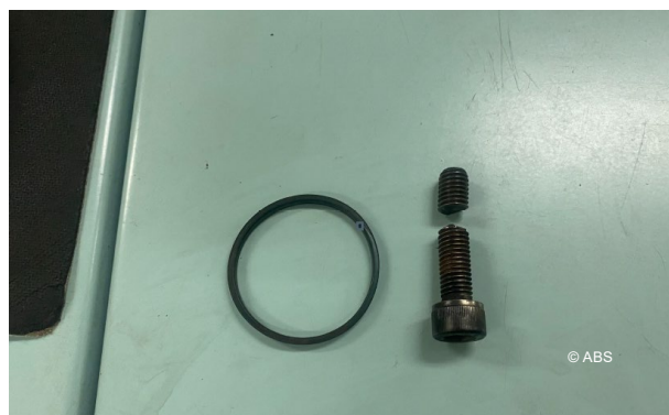
ME Cylinder injector found with broken hex bolt
