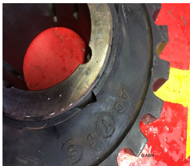
Emergency generator coupling worn
